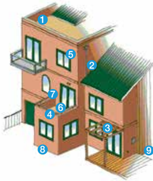
Common risk areas in a house. Elements numbered on page 16. Source: BRANZ Weathertight.
